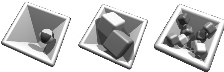
Fig. 7.10 Contact dynamics between a ball, boxes and funnel. The boxes and the funnel are represented by triangularized shapes
